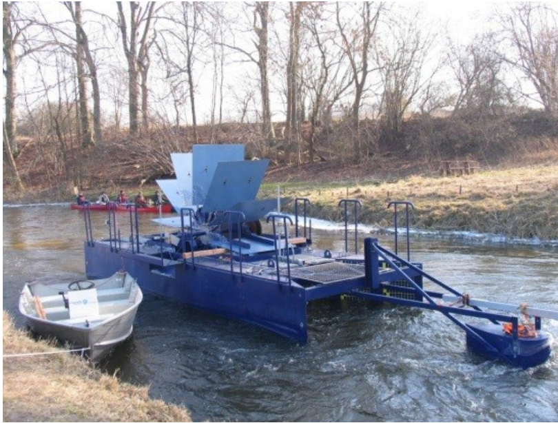
Fig. 5.3: Free Stream Energy Converter in the Warnow River
